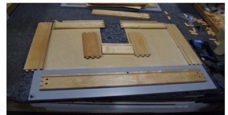
11. Apply glue (optional) to the drawer head and attach the left and right drawer box sides to the drawer head and tap the dovetails into place using the mallet. (Note: The drawer box front for the top drawer ONLY is pre-attached to the drawer head).
