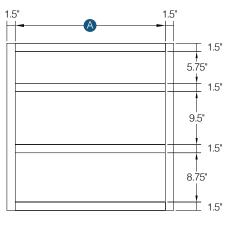
**Outer Dimensions Top Opening Top Drawer Front** Item Code Size w н Α D н н Α DB12-3 12" 34.5" 24" 9" 5.75" 11.5" 6.75" 34.5" 12" 5.75" 14.5" 6.75" DB15-3 15" 24" DB18-3 34.5" 6.75" 18" 24" 15" 5.75" 17.5" 23.5" DB24-3 24" 34.5" 21" 5.75" 6.75" 24" DB27-3\* 27" 6.75" 26.5" 34.5" 24" 24" 5.75" DB30-3 30" 29.5" 6.75" 27" 5.75" 34.5" 24" DB33-3\* 33" 30" 5.75" 32.5" 6.75" 34.5" 24" DB36-3 36" 34.5" 24" 33" 5.75" 35.5" 6.75"
